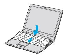
10 Close the computer cover, then tighten the screws on the bottom of the computer.
